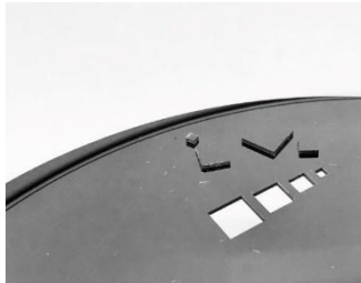
Precision Laser micromachining of Si wafer.
